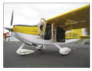
the aircraft is so much as rolling forward, there's enough rudder authority for gentle turns without brakes. Takeoff is with 20 degrees of flaps and requires little rotation once the wing is at flying speed. We were several hundred pounds under gross on our test flight so we climbed just over 1500 FPM.
