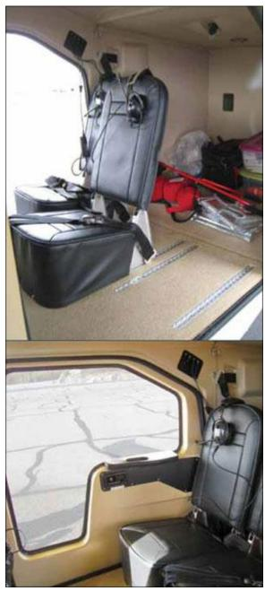
The E350's split personality is evident the moment you enter the cabin: Four huge doors with observer windows access a 53-inch interior sporting three quick-release seats in back. While the interior isn't opulent, the fit and finish quality is on par with any major aircraft manufacturer.
